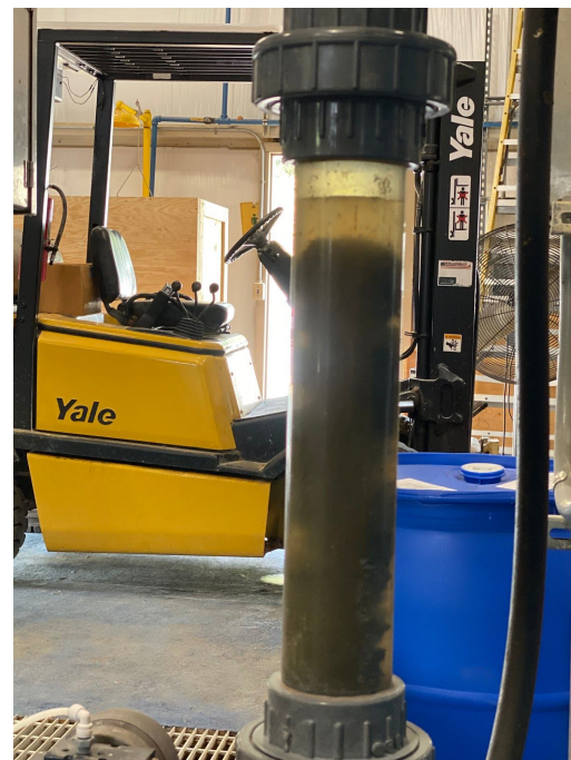
Figure 4. Biosolid flocculation with polymer
