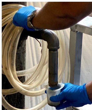
Figure 33. Biosolid sample after secondary digestion
